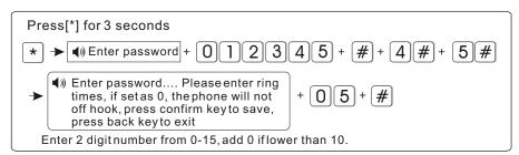
Note: The max. Ring times as per the local communication, if set 0, not off-hook.
