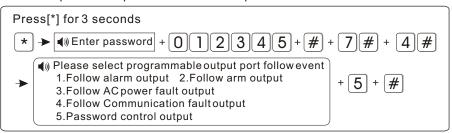
Hint: when setting as password control output, press key 5 for 3 seconds, then enter the user password, the programme output port will be open or closed. Voice phone or SMS also can open or close the outport.
