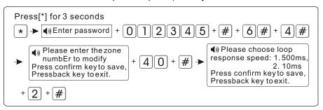
Note: Normall the detector's response speed is 500 millisecond, high speed response detector like vibration detector is 10 millisecond
