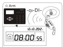
Press the keyfor arm away on remote or the keypad, then you hear "system armed, please exit the protection area" there will be "Dee-dee" sound to confirm the system is armed successfully.
