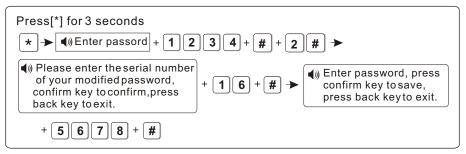
Note: Can set 16 user passwords, corresponding password No. from 01 to 16, Only No.1 password can enter user setting.
