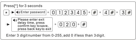
6.4.4 Set siren time: The siren ring time after alarm is triggered (the default setting is 5 minutes)
