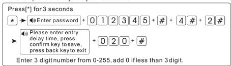
Note: Entry delay is just effective for delay zone. Other zone types can't enter delay.
