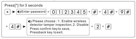
6.4.9.5 Set force arm: if enabel set force arm, when there is zone trouble, the system can be armed and report the trouble zone's bypass message to CMS. If disable the force arm, the system can not be armed (factory default is disable forem arm)
