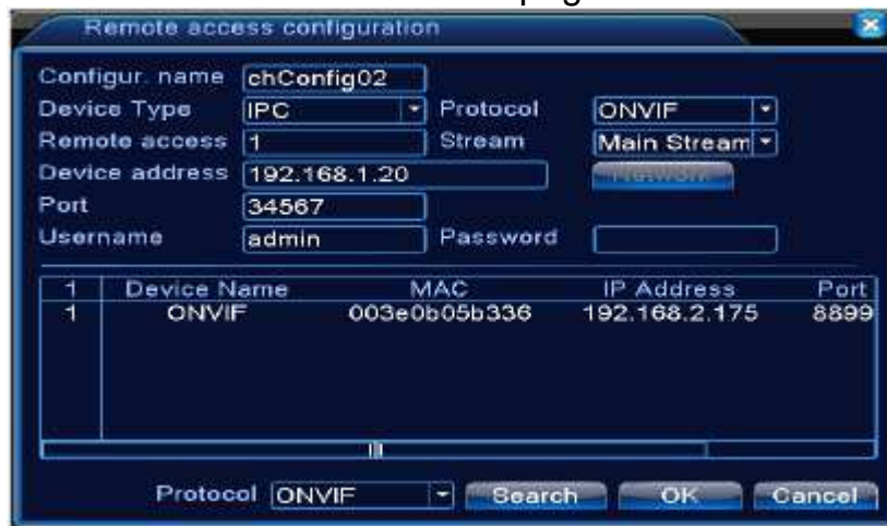
Figure 4.36 Remote Access Configuration
