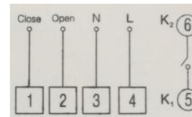
wall-hung boiler wiring diagram
