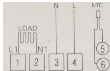
Electric heating wiring diagram
